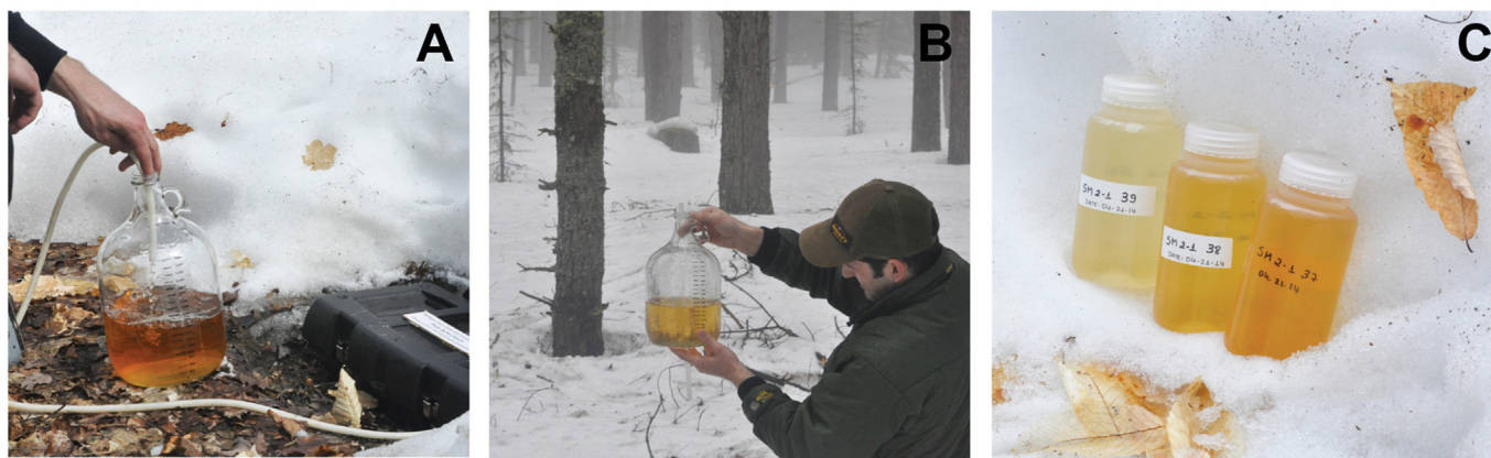
Fig. 9. Photos showing soil water sampled during spring snowmelt, 2014. A. Water being pumped from the buried bottle, into a glass collection bottle. B. Determining the content of the leachate in the bottle. C. Comparison of soil water recovered from lysimeters beneath the (left to right) B, E and O horizons of a soil. Note the yellow-brown colors of the leachate, rich in DOC, in all the photos. Water leaving the B horizons in summer and early fall typically shows no yellow color at all. (For interpretation of the references to in this figure legend, the reader is referred to the web version of this article.)
